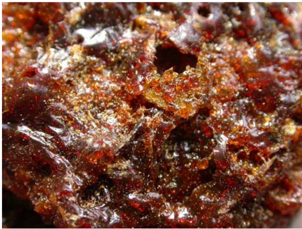
Fig. 2 Melted surface of a specimen which was released hot from the experimental arrangement, so there were liquid parts which hardened in air under ambient conditions. Inside the material is porous but still tough. The area shown is about 20 mm wide
